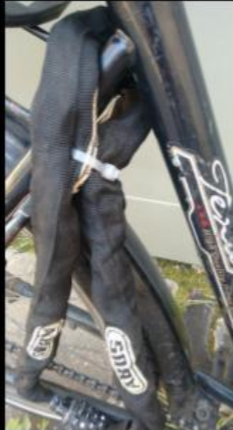
Chain lock secured through frame using cable ties to ensure bike is locked through frame
